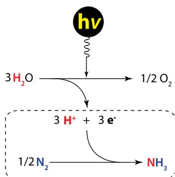
*Scheme for an artificial "Solar-to- $NH_3$ " system in which a solar-driven water splitting reaction provides proton and electron equivalents for the fixation of  $N_2$ . The reaction shown within the dashed lines is the subject of our work*
