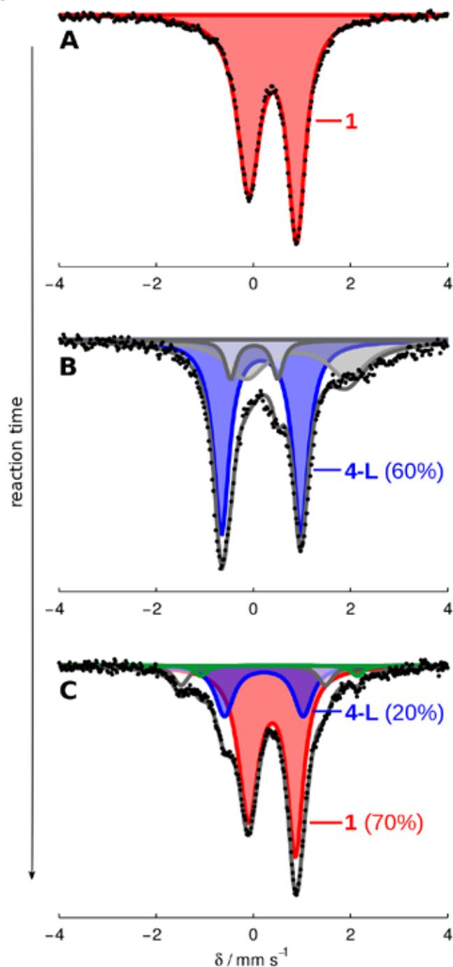
*Time resolved Mossbauer spectra of a catalytic reaction mixture, showing the conversion of precatalyst (red) into hydride resting state (blue) under active turnover, and regeneration of precatalyst (red) from hydride (blue) at longer times.*
