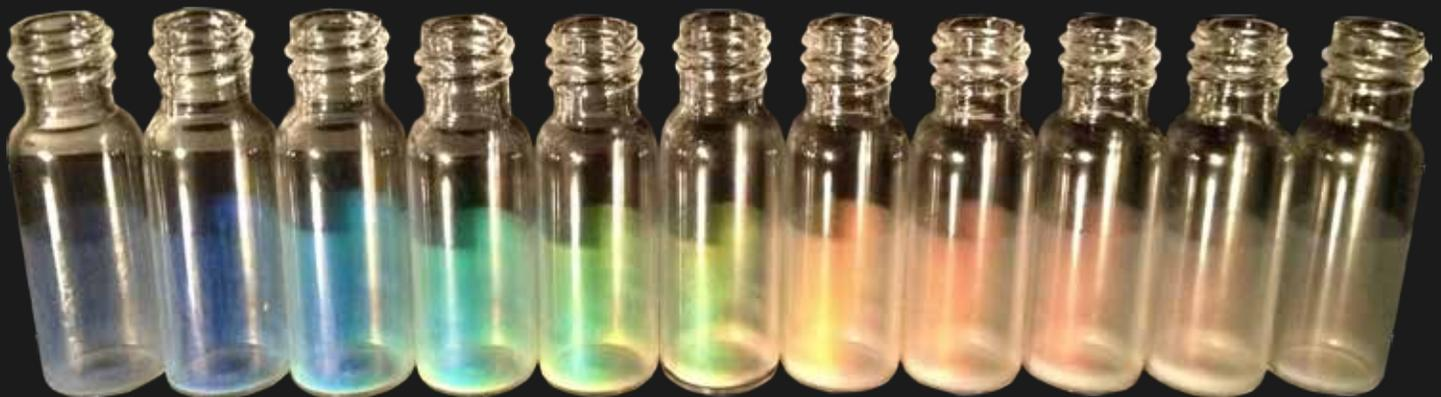
An array of polymer photonic crystals, synthesized by blending the two samples on each end together in different ratios.
