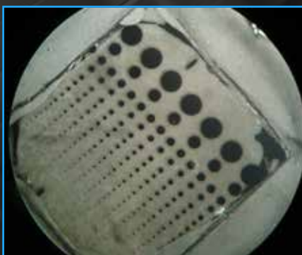
150 dots of ceramic catalyst \text{La}_{0.5}\text{Sr}_{0.5}\text{CoO}_{3-\delta} on a 5 mm x 5 mm substrate
