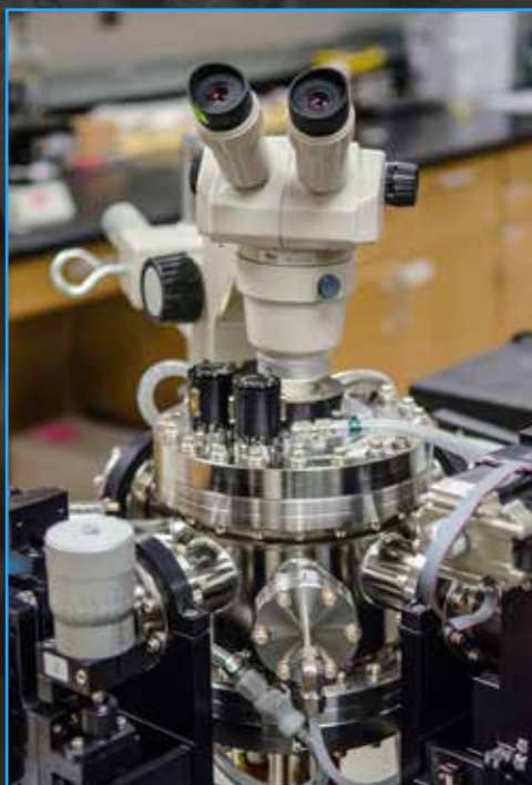
Custom automated impedance microprobe developed for this project.
