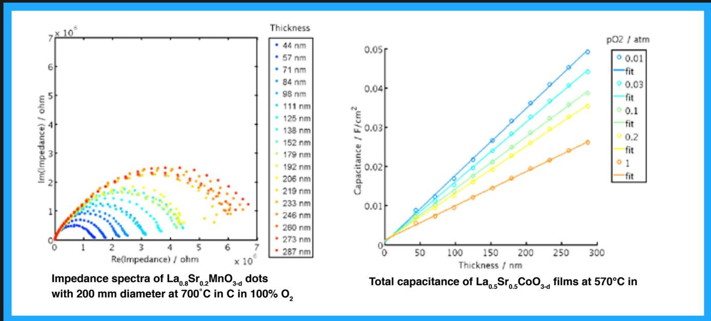
The impedance microprobe is now online and rapidly measuring hundreds of catalyst dots under realistic fuel cell operating conditions, using systematic variations of several [experimental variables](#) to quantify fundamental [material parameters](#):
