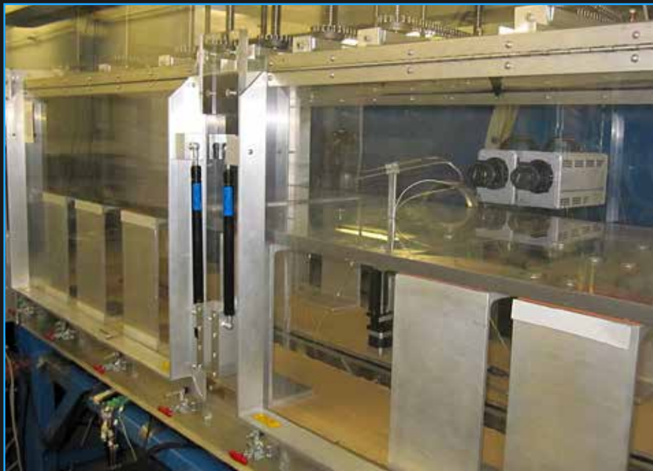
Image showing the test section of the Merrill wind tunnel at Caltech where experiments on perturbed turbulent boundary layers are carried out.
