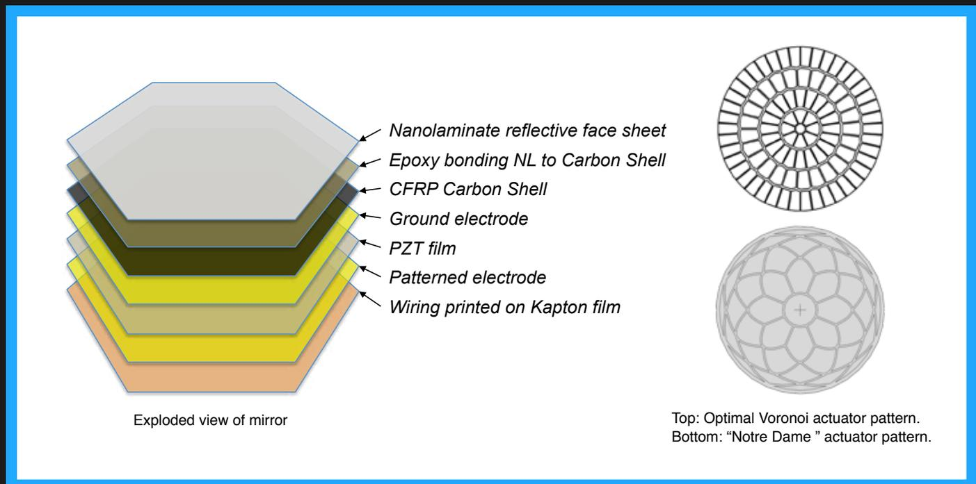
The pattern of actuators plays an important role in improving the shape-correction capability. We have developed two optimization approaches. The first approach treats the actuator pattern as a Voronoi tessellation and optimizes the tessellation through an evolutionary algorithm. The second approach uses an intuitive "Notre Dame" actuator pattern to correct the asigmatism error, which is one of the dominant optical aberrations for our thin mirrors.
