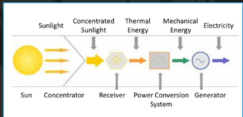
Schematic of a CSP system per [www.csp-world.com](http://www.csp-world.com)
