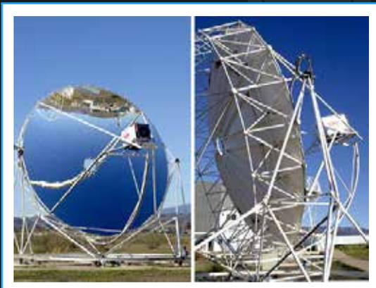
Parabolic dish concentrator. (Courtesy of PSA, Spain)
