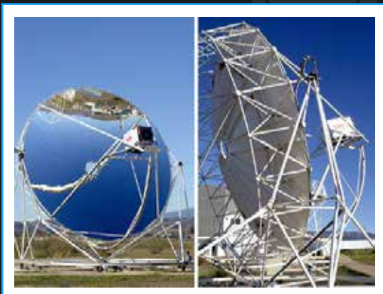
Parabolic dish concentrator. (Courtesy of PSA, Spain)
