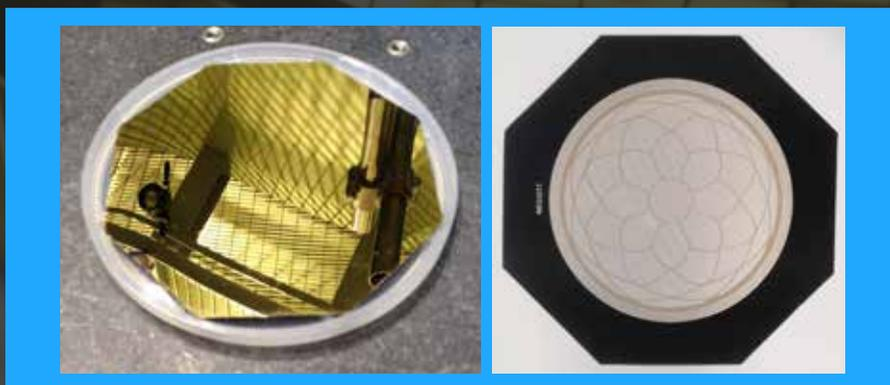
A 150-mm-diameter prototype with a highly reflective layer on the front side (left)
