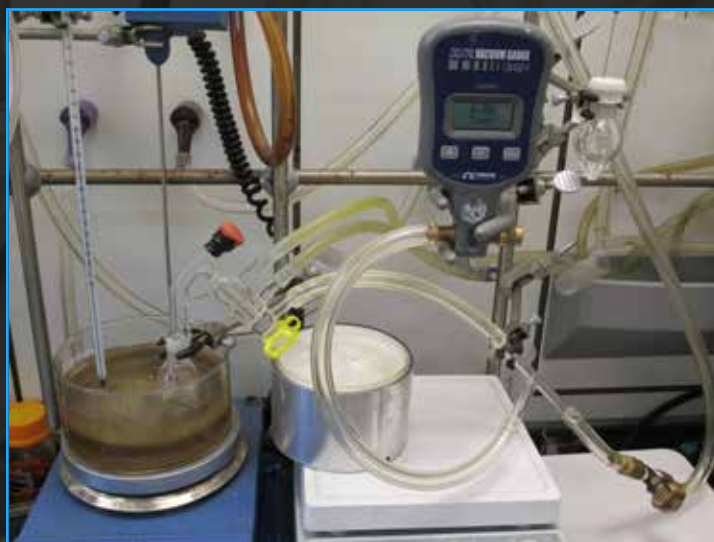
The reaction is carried out in a vacuum distillation apparatus. The volume is small since no solvent is needed.
