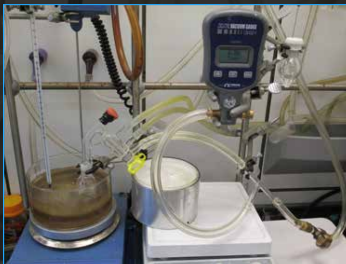
The reaction is carried out in a vacuum distillation apparatus. The volume is small since no solvent is needed.
