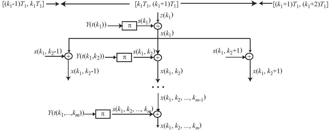
Figure 3: Dispatch policy  $\pi$  selects  $s(k_1, \dots, k_j)$  as a function of  $Y(t(k_1, \dots, k_j))$ .
