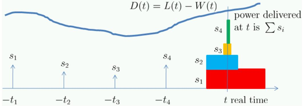
Figure 1: Power block  $s_i$  is purchased  $t_i$ -ahead of real time  $t$ ; net demand is  $D(t)$ .
