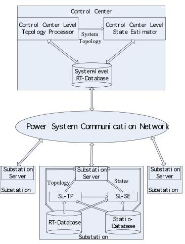
SL-TP: Substation Level Topology Processor
