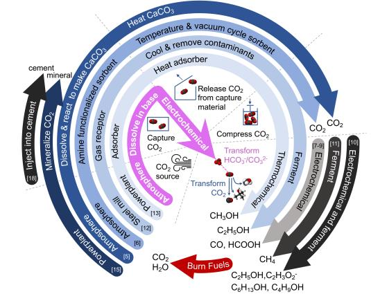
Schematic of steps for various prototype systems which capture and/or convert  $CO_2$ . The blue arrows represent processes that capture and convert  $CO_2$ , grey arrows represent processes that only convert  $CO_2$ , and the pink arrow represents the process that we propose.
