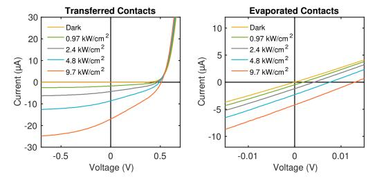
Transferred-contact devices show diode-like IV curves and open-circuit voltage > 500 mV. Evaporated-contact devices show resistive IV curves and open-circuit voltage below 15 mV.
