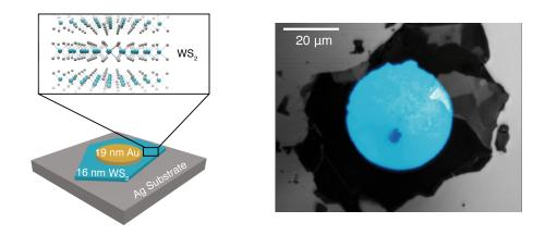
Ultrathin (<150 nm) solar cells made from 2D semiconductors with transferred contacts. Left, schematic. Right, photogenerated current mapping.
